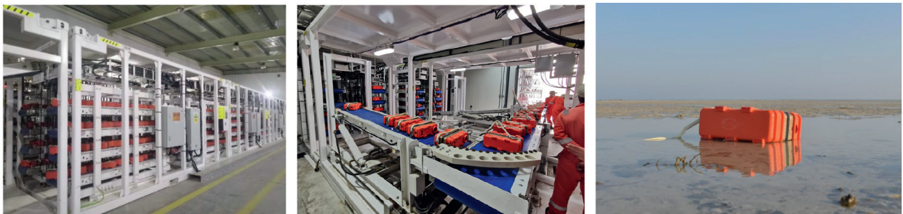
Figure 6 Field context: (left and centre) GPR300 on LARS (launch and recovery system) ready for deployment, (right), A node laid out and anchored on the foreshore.
