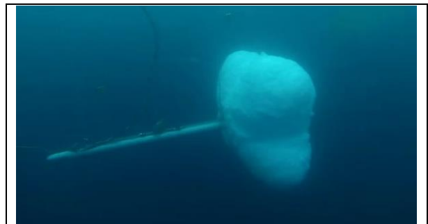
Figure 2: The new source just after firing. The maximal bubble radius is almost 2 meters. To indicate the scale, note that the length of the 26,500 cui source that is visible to the left in this picture is 7.3 m.
