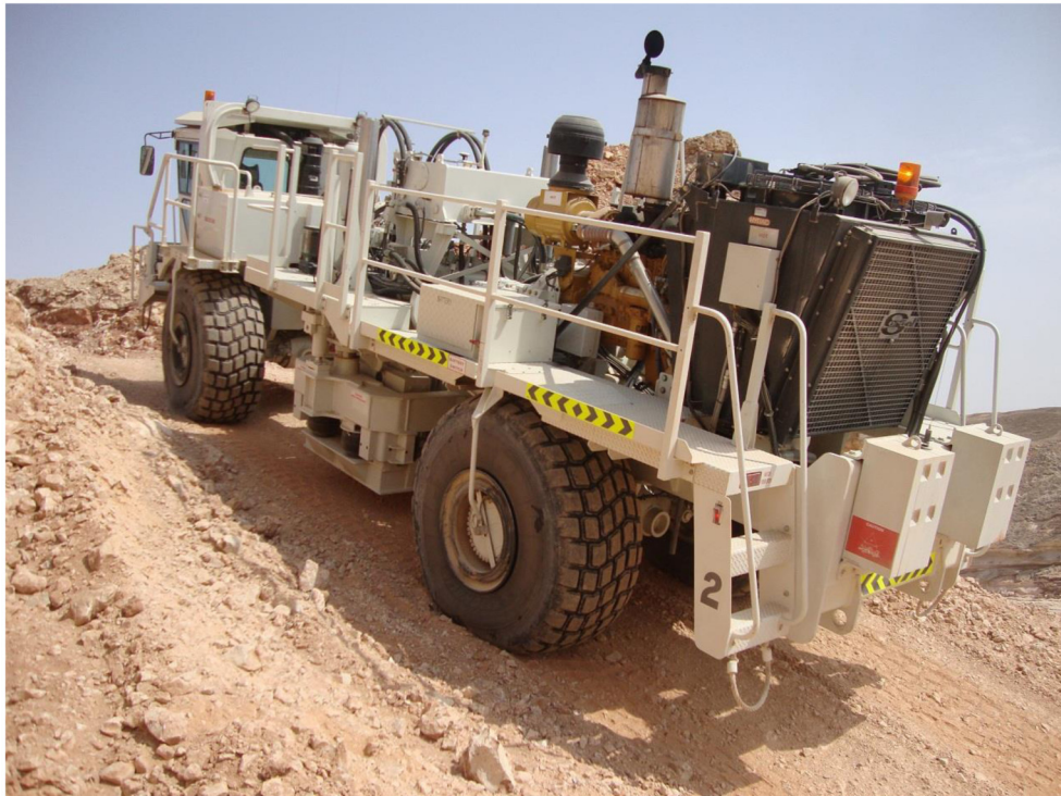
Figure 6—Super-heavy vibrator in one of the project's steep area
