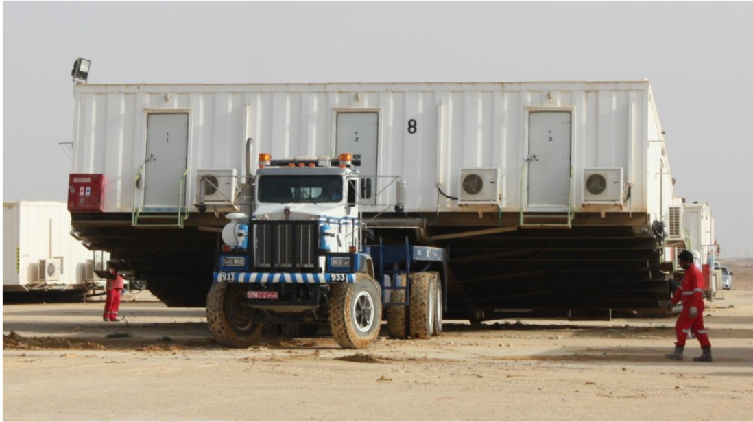
Figure 7—Base camp move, optimized by the use of 40 by 40-foot mega-skid. Each skid is around three times the size of a standard skid and can accommodate the 50 senior staff kitchen and mess or 24 staff in individual cabins
